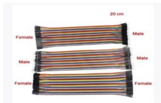
Figure 7: Jumper wire types
